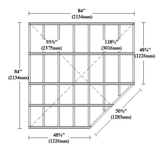
NB:- Floor joists run from right hand back to left hand front. Optional Floor Bearers run from left hand back to right hand front.
